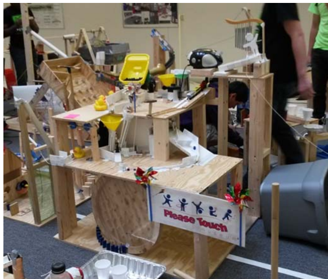
Fig. 1. Example twenty-nine event Rube Goldberg Machine from Spring term 2014 pilot section. Machine begins at top right, near wind-chimes, and ends at left near rubber duck. Events travel along multiple levels, traveling both upwards and downwards. Machine is approximately 1m wide by 1m deep, and 1.5m tall.
