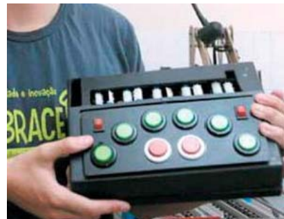
Fig. 8. The prototype of the braille phone, a mobile phone for blind people designed to send messages in braille.
